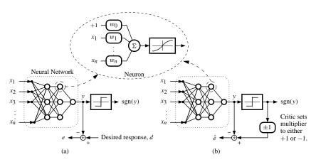
Figure 2. Multilayer neural network: Adapted (a) using backpropagation; (b) using critic.
