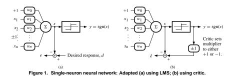
and *W* are the weight values of the neuron. (*X* is augmented with a bias value of 1, and *W* is likewise augmented with a weight to multiply the bias value.) When a desired response is available, an error signal may be computed and used with the LMS algorithm to update the neuron's weight values:  $\Delta W = 2\mu eX$ , where e = d - s is the difference between the desired response and the neuron's internal sum, and  $\mu$  is a small positive constant that controls the learning rate.
