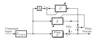
Figure 5: A system which is unbiased by disturbance.
